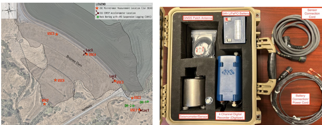
Fig. 6 (a). Location of the microtremor measurements on Briones Dam, (b) The sensor setup includes the Pegasus digitizer, connecting cords, and a battery.
